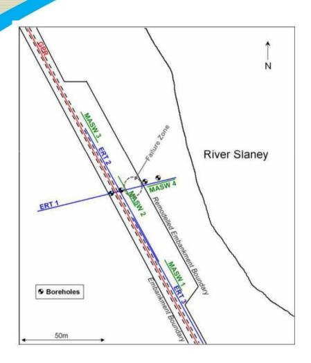
Resistivity investigation across failure plane and along track to confirm soil stratigraphy and investigate suspected lateral flow of water along embankment
