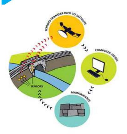
WP1 aims to bring about a step change in the traditional methods of visual inspection and ad-hoc monitoring with integrated monitoring systems which utilize the latest embedded sensor technology and optimized in-situ testing methods.
