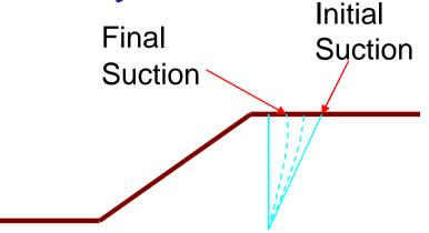
As rain falls, suctions reduce. A wetting front develops as the ground becomes *almost* saturated from the top down
