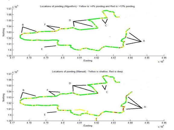
Comparison between automated (top) and manual (bottom) water ponding analyses for a 26km site close to TRL in the UK
