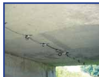
Strain gauges on a bridge deck
