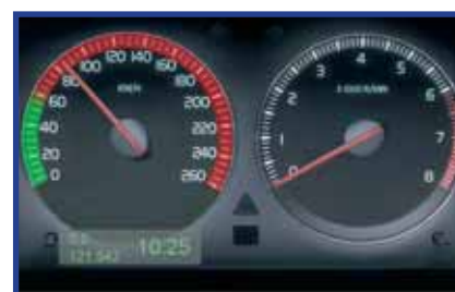
Figure 1. Recommended speed interface used in the driving simulator study
