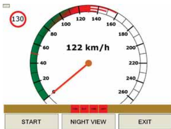
Figure 4. Driver low friction warning system with recommended speed (Pilot 2)
